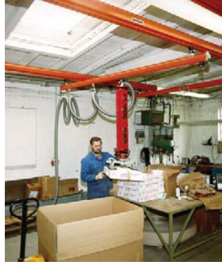
A workstation crane fitted with a balancer and a vacuum lifter for handling large or heavy containers
